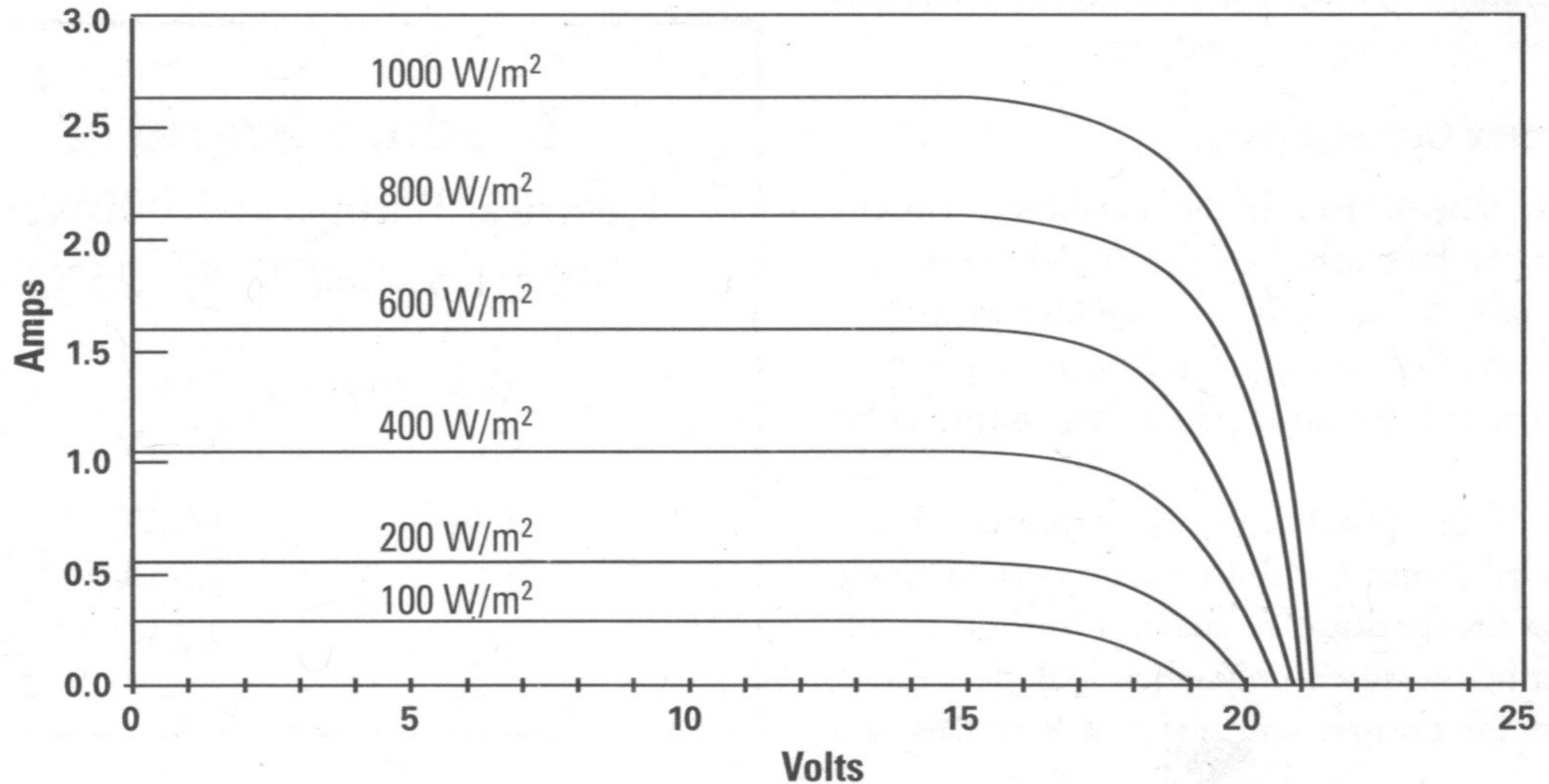
The more sunlight falling on a panel, watts per sq. meter, the more amperage
