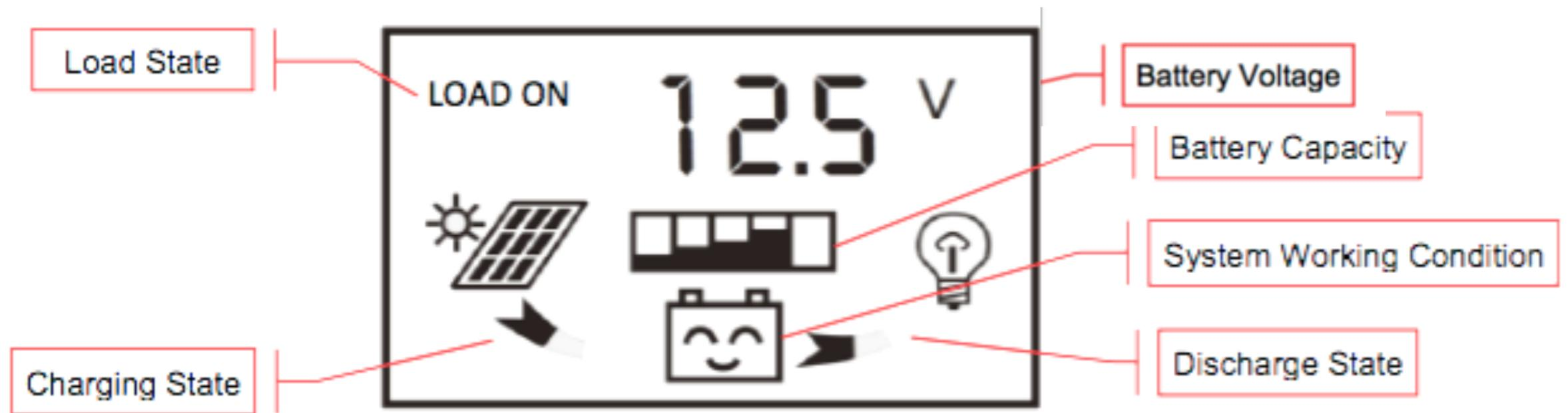
The Main Interface displays the current state of the Load, PV charging, Load discharging, battery capacity, and overall system working condition.
