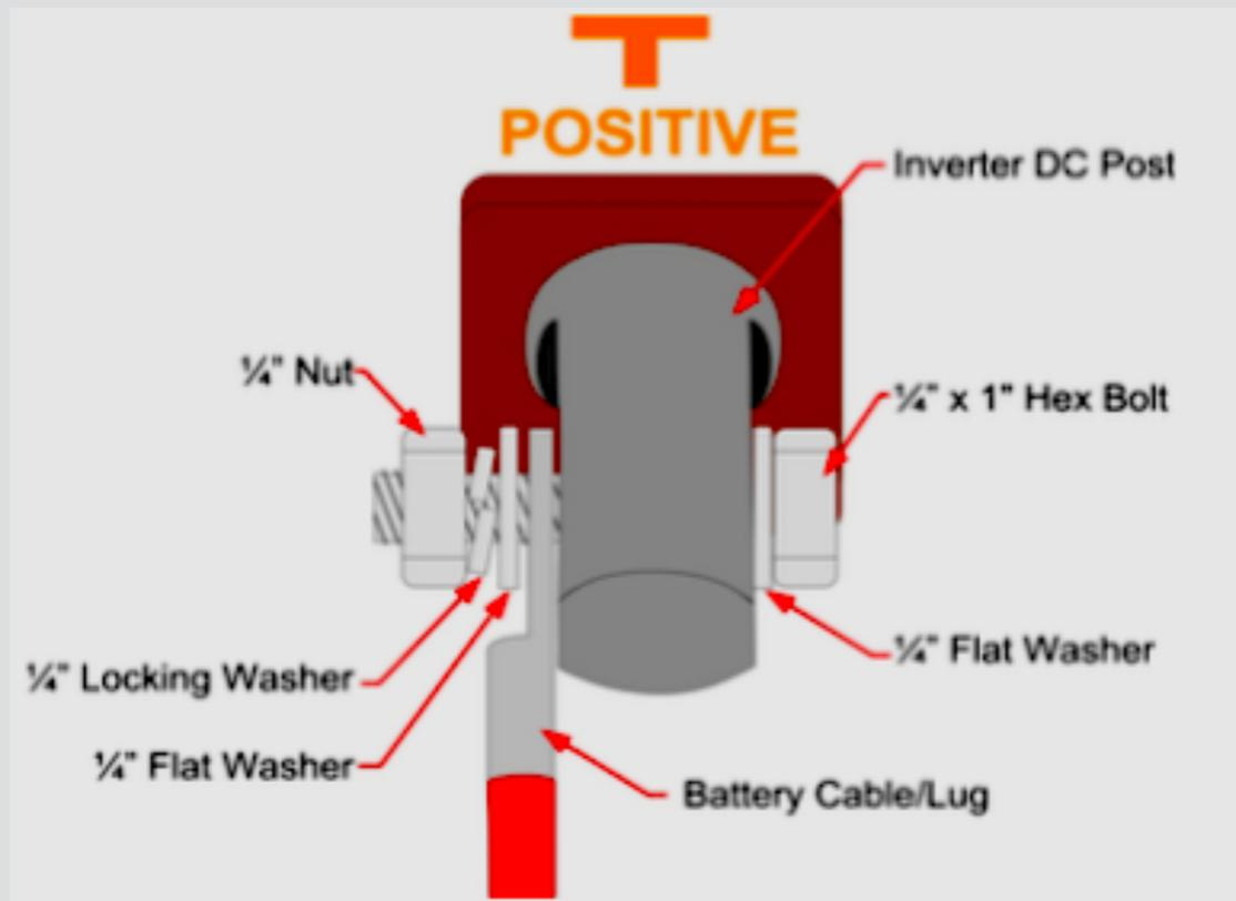
The VertaMax has two DC terminals, one positive and one negative. Red is Positive [+ ] and black is Negative [- ] and has the same polarity as the battery. When connected, positive must connect to positive (red to red), negative connect to negative (black to black)
