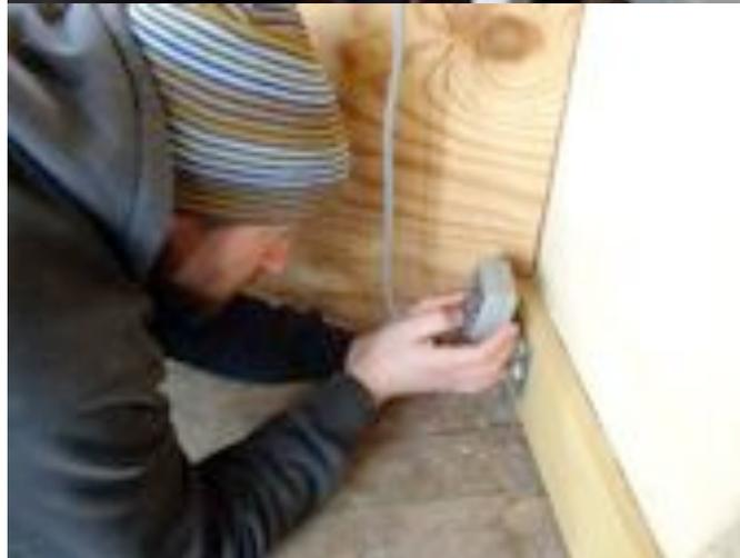
*He attached a Kill-A-Watt watt-meter to measure the amount of electricity the refrigerator was using in real time.*
